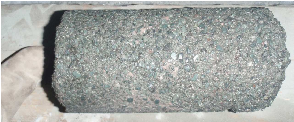
Photo 10: Drilled core was taken around station 1+60 on the downstream (HB12-ND-CORE-DC73-20120311). Note that the very bottom of the core was noted to slightly melt when cored. This is expected to have resulted as the core was taken immediately after a -2C reading was obtained. This north area is expected to be placed on during dayshift tomorrow.
